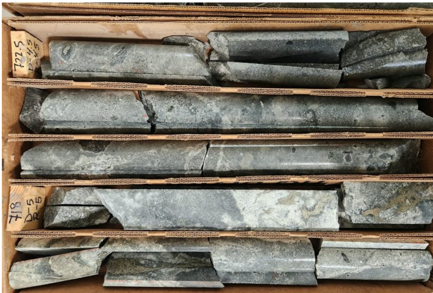
Figure 3: Photo of altered, pyrite-bearing diorite at 218 meters in EC-11.
