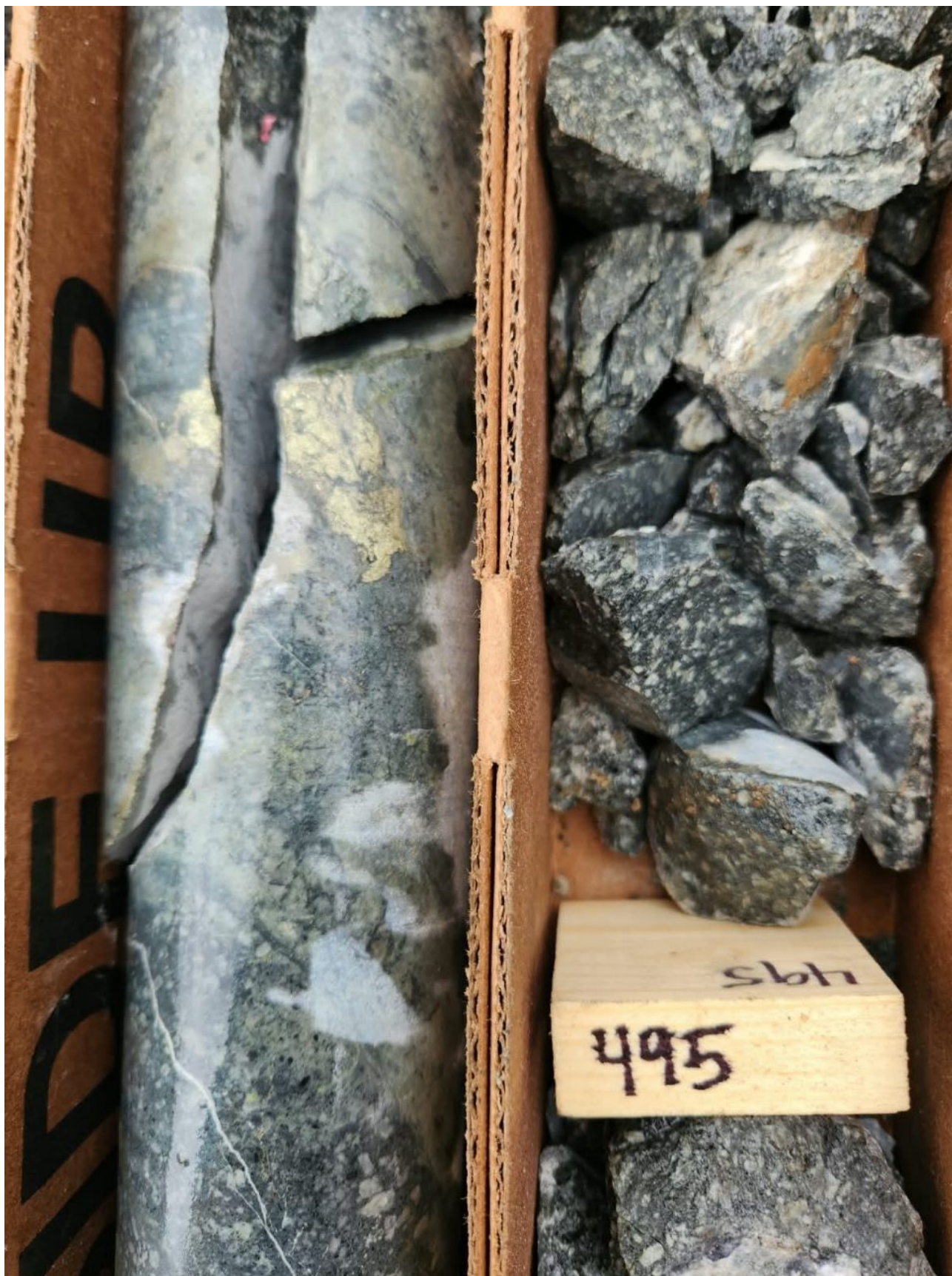
Figure 1: Photo of altered, pyrite-bearing diorite at 151 meters in EC-10.
